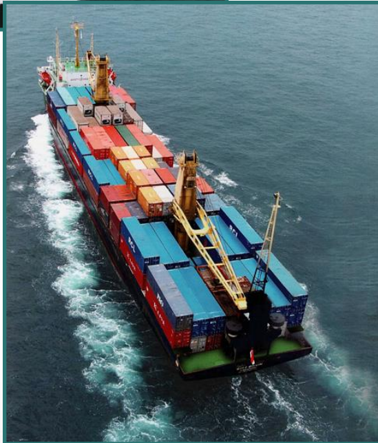
M.V. Wana Bhum (2) 24,100 T - 2378 TEU - 2005 Main Engine: MITSUBISHI 7UEC68LSE 20580 KW (27900 PS) 95 RPM
